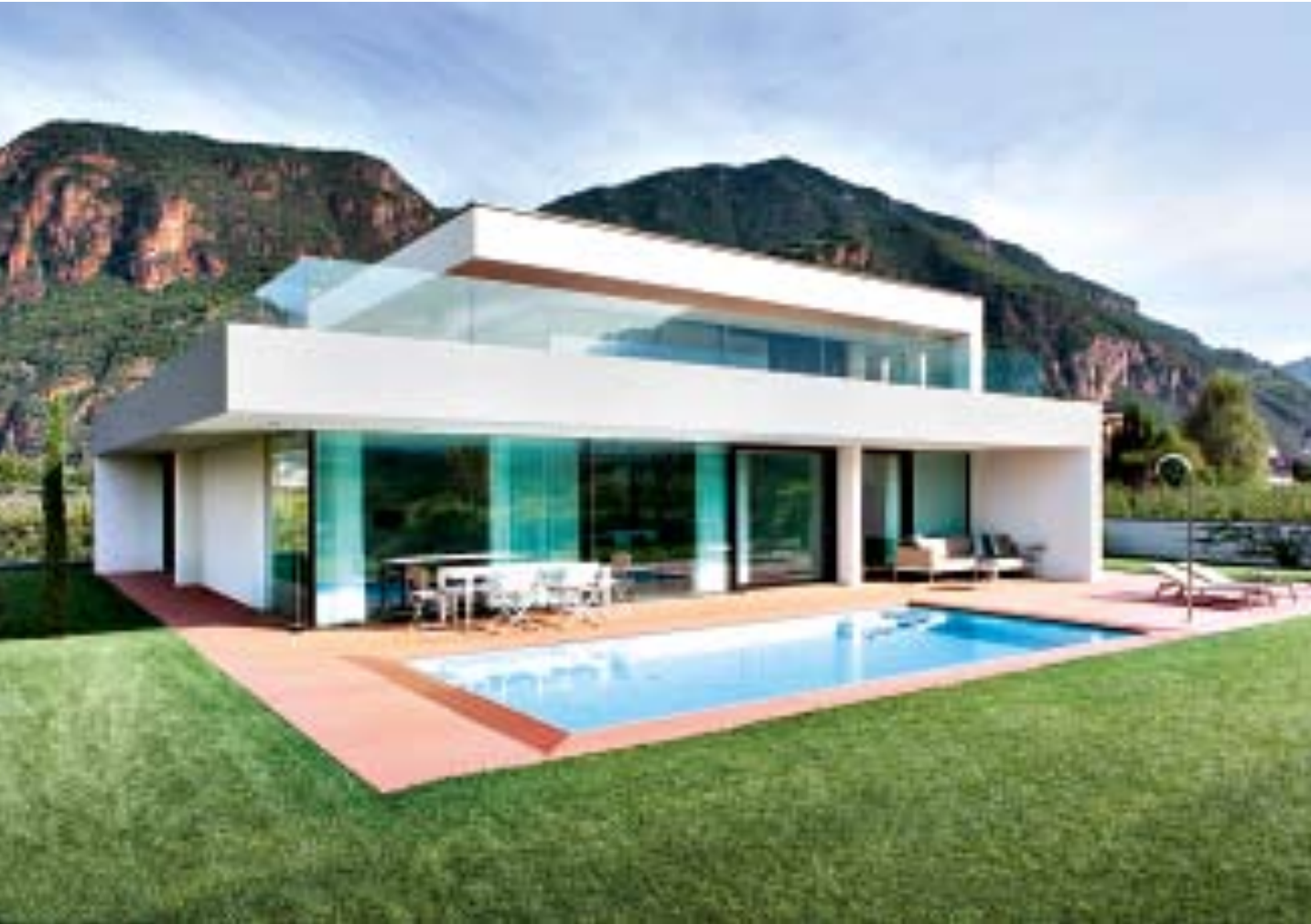
The building’s distinctive features are its cantilevered roofs, which protect the fully glazed rooms from excessive sunlight in the summer.
